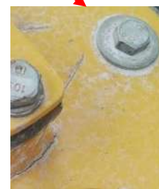
Fatigue cracks of the fuel tank
