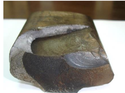
Change in the direction of horizontal crack propagation
