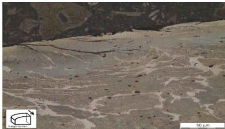
Cracks initiation at rail surface after 5.3 and 10.6 MGT
