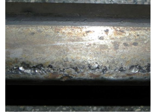
Change in the direction of horizontal crack propagation
