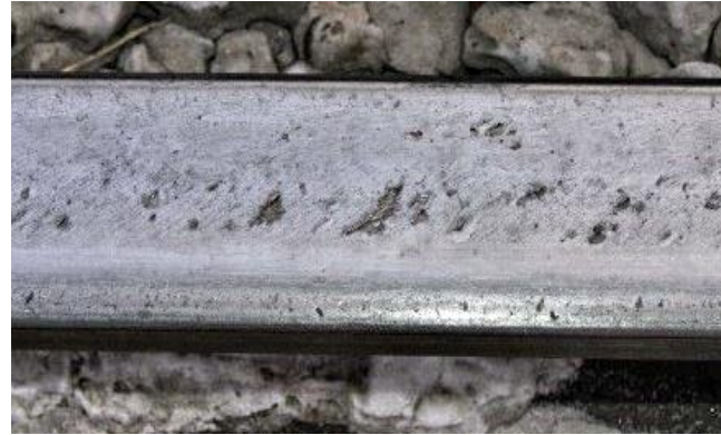
Head checks on rail running surface
