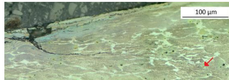
Cracks initiation at rail surface after 5.3 and 10.6 MGT
