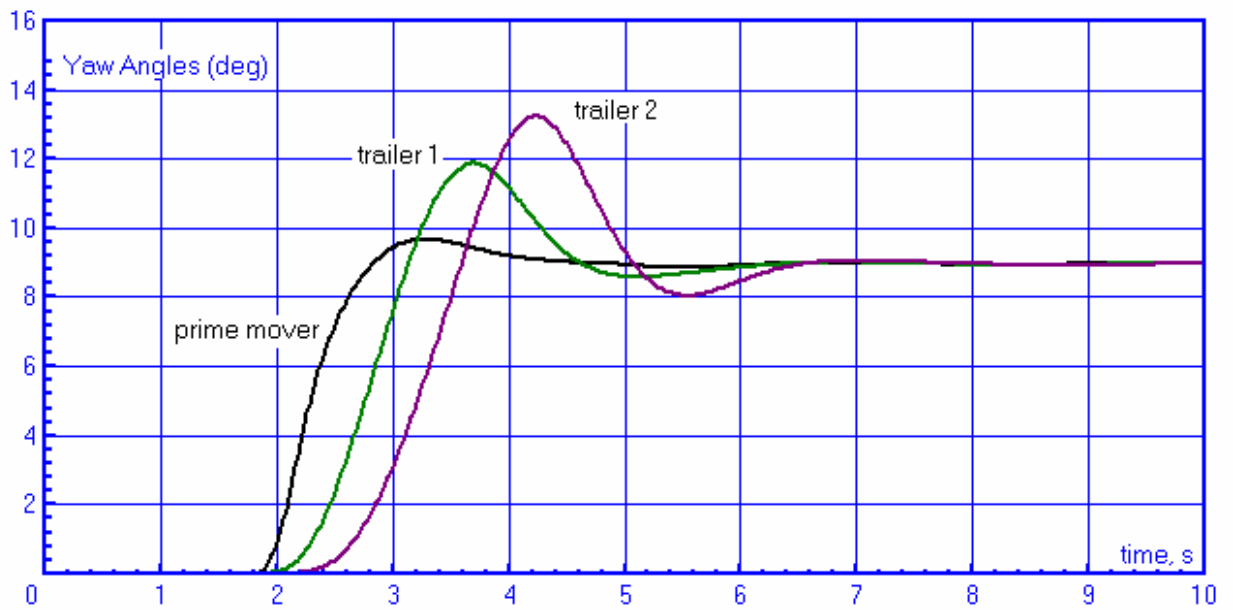
Figure 5.7. Yaw angles from B-double pulse steer simulation Corresponds to Fig. D1.1(h), page 74 in [1]
